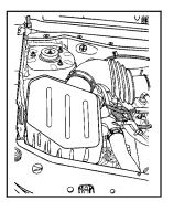
1. Unscrew the clamp on the air duct hose.
